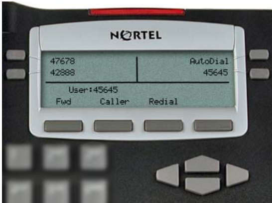
Figure 5: Logged on to an IP Phone 2002
